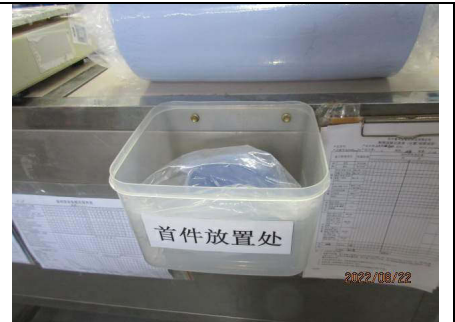
Photo 15) First piece sample provided at vulcanization molding area
