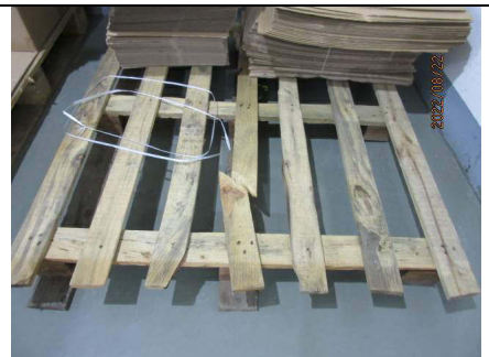
Photo 65) NC 4.8.6 Broken wooden pallet was used at packing area
