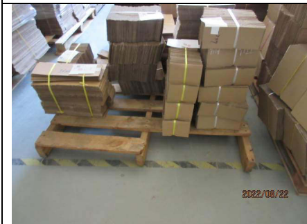
Photo 64) NC 4.8.6 Broken wooden pallet was used in raw materials warehouse
