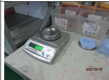
Photo 67) NC 7.3.1 Electronic balance (number 207) used for color powder weighing was not calibrated in time
