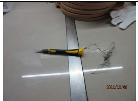
Photo 62) NC 4.8.3 One blade was not fastened to workbench at injection molding area
