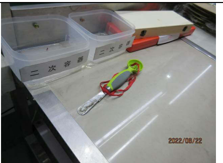
Photo 63) NC 4.8.3 One sharp tools used by inspector at assembly and packing workshop was not fastened to workbench
